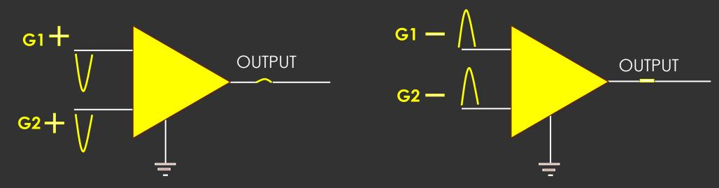
When the inputs are the same or close to the same, the output may be 0 or minimal. This is also sometimes called "equipotential" meaning equal to potential.
